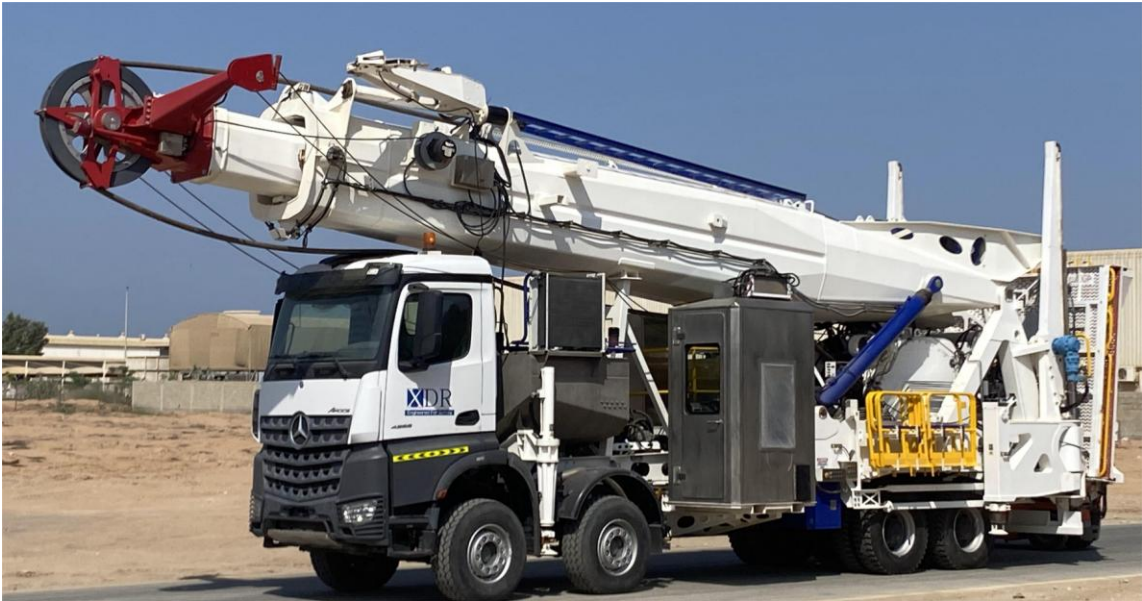
XDR 250 Rig mounted on a custom Mercedes Arocs 4858 580hp. SIL 2 Rated
